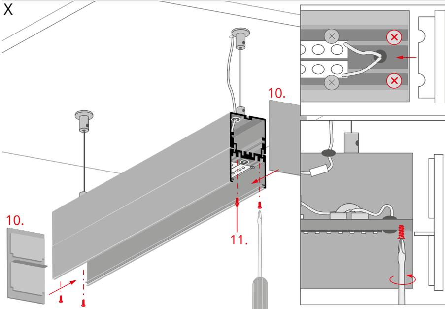
Insert the end cap bolts (11) in threaded channels (as shown in the figure).
