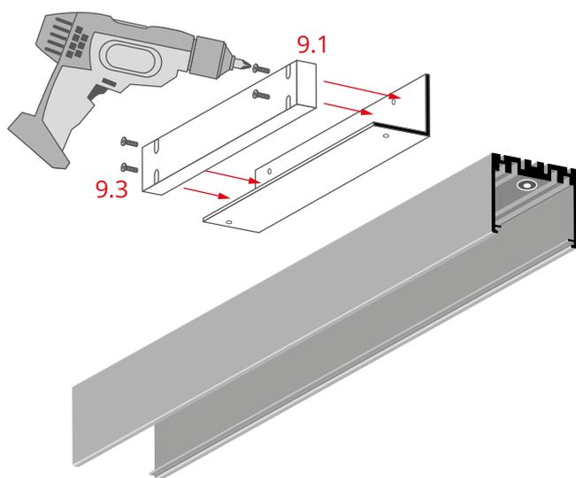
Mount the power supply (12 V / 24 V) (9.1) to the insert with bolts (9.3).
