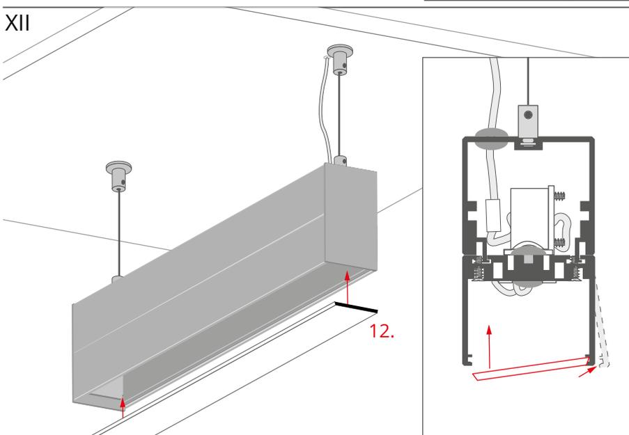
Attach the cover (12) by slightly bending the edge of the profile outwards.
