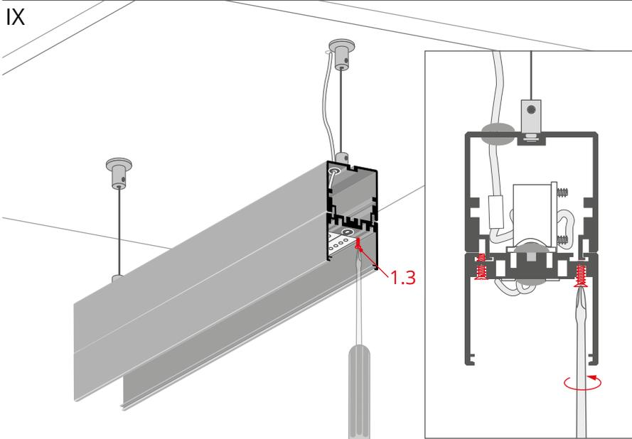
Secure the profile items against slipping out by tightening the locking bolts (1.3), embedded in the pre-drilled holes.
