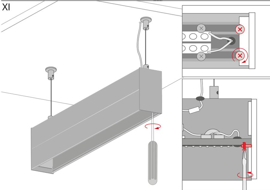
Lock the end caps by tightening the bolts (the end cap has bolt holes in the inner flange).
