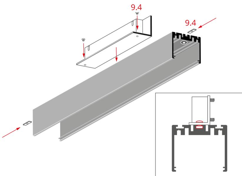
Attach the insert to the profile with the connector (9.4).
