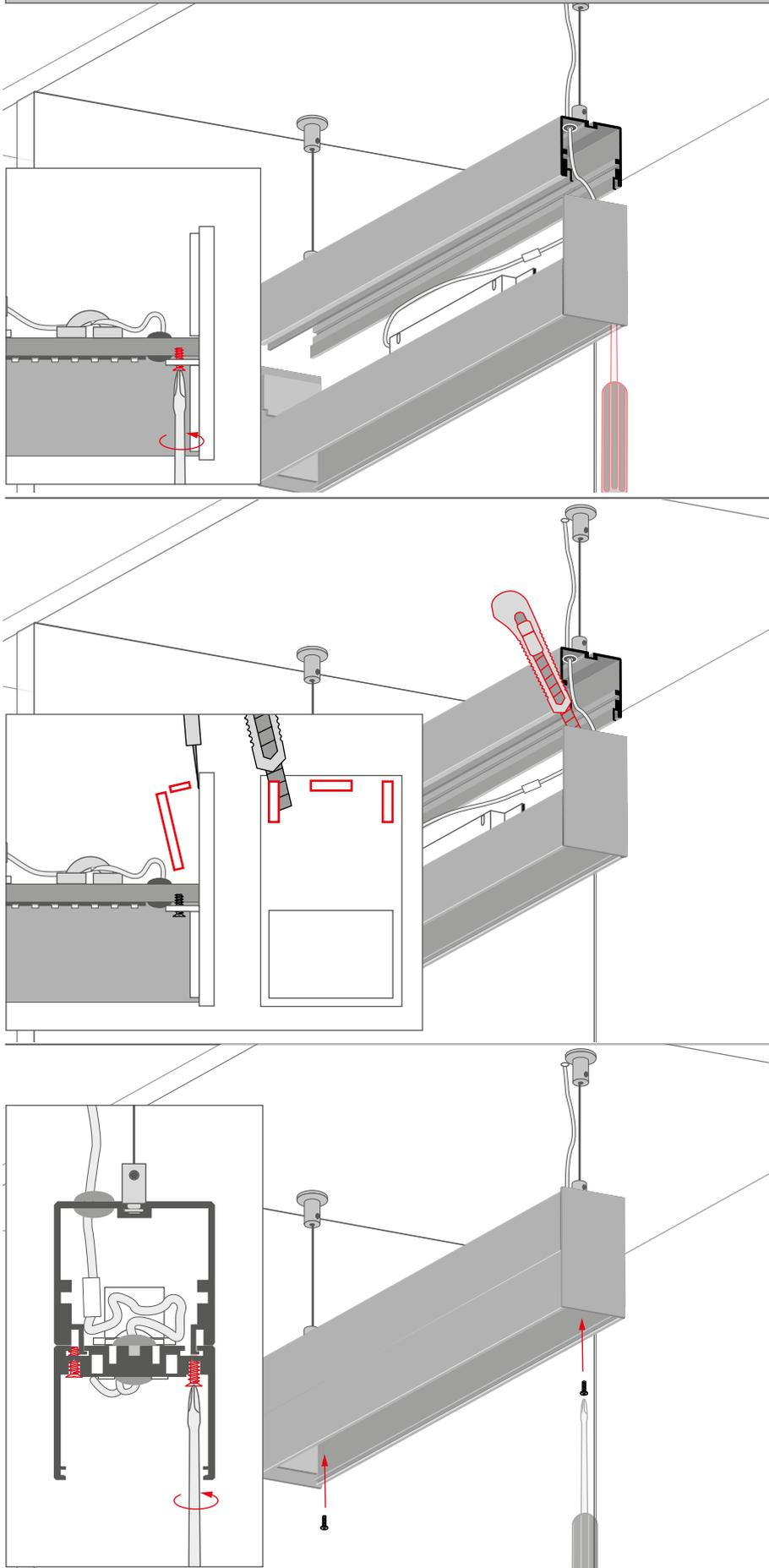
In case of „wall-to-wall” installation it is necessary to mount the fixture with the end caps from the bottom.
