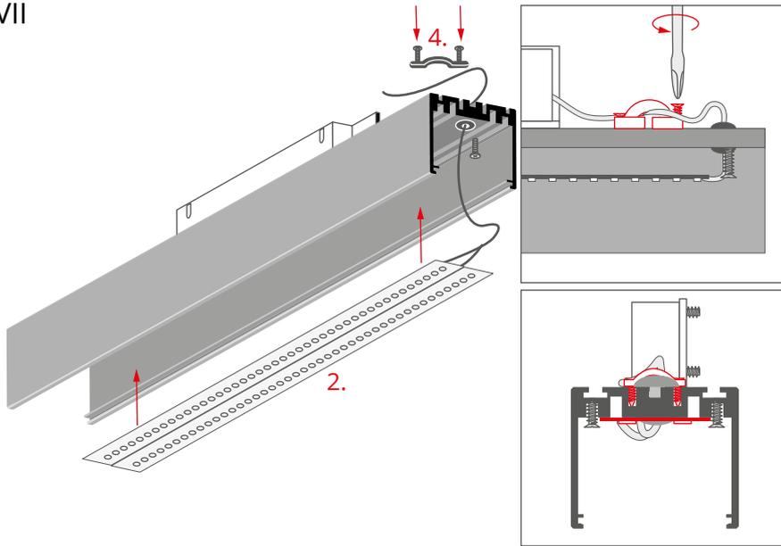
Adhere the LED tape (2) into the profile item (1.2). Run the power cable through the gland.
