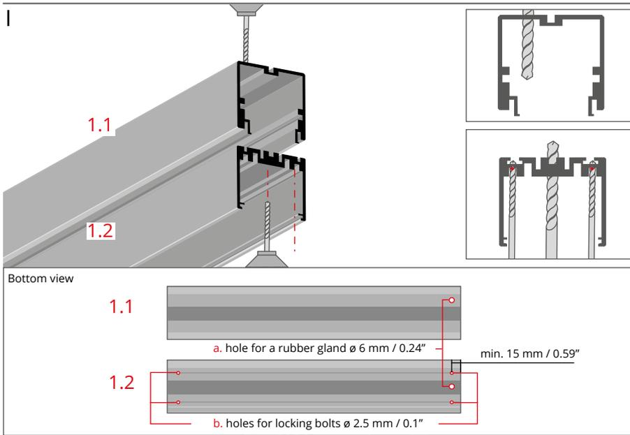
a. Drill holes for the glands in the profile items (1.1,1.2). Drill holes in the places in which you want to put the power cables.
