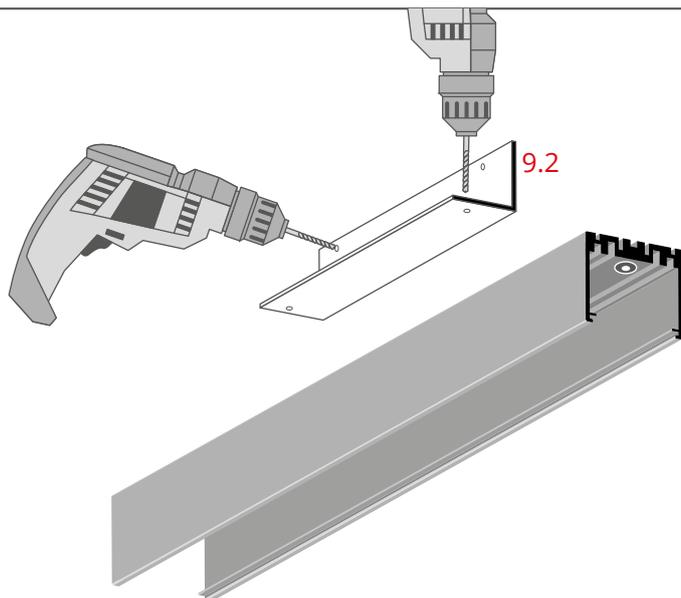
Drill the holes for bolts and connectors in the insert (9.2).
