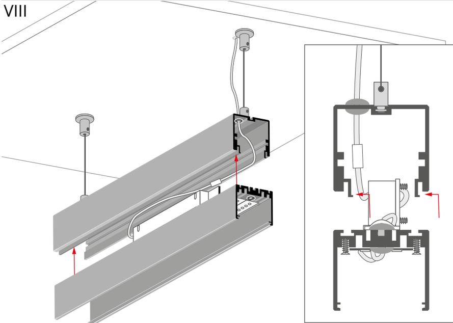
Connect the power cables. They can be placed in the chamber inside the mounting strip.
