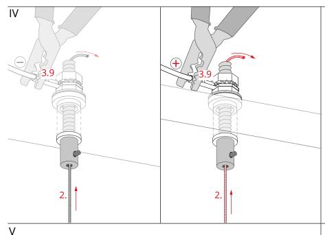
Lead the steel cables (2) through fastener bodies and threaded sleeves to the other side of the fastener.
