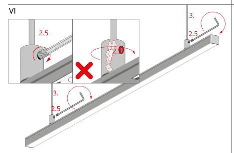
Insert the rods (3) into the holes in the heads of the fasteners. Lock them by tightening the pressure screws (2.5) with an Allen key.
