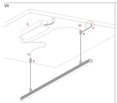
Suspend the lighting fixture from the ceiling fasteners (4), connected to the power supply (12 V / 24 V) (5).
