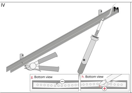
Cut the wires to a length that is convenient for you and solder to the LED tapes (figures g, h).
