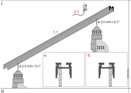
Drill wire holes (2.1) in the profile (1.1). Drill the holes right next to the profile wall so as not to damage the upper edges of the channel on the profile's back (figures a, b).
