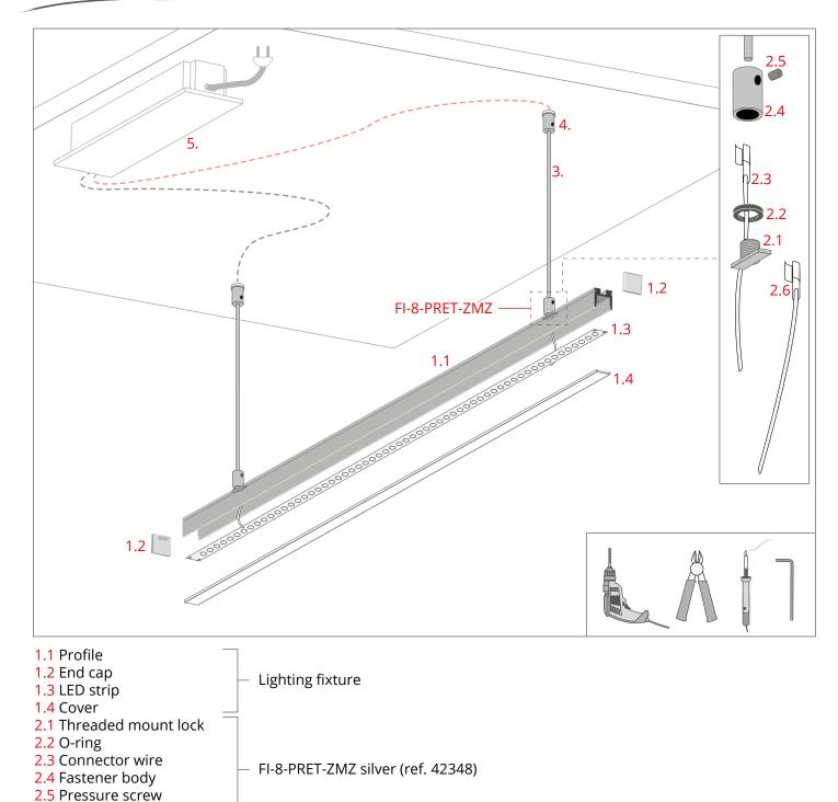
**NOTE!** All LED tapes must be connected to a 12 V or 24 V power supply.
