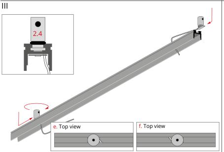
Run the connector wires through the holes and slide the fasteners into the channel on the back of the profile. Move them as close as possible to the holes and lock them by tightening the heads (2.4, figures e, f).
