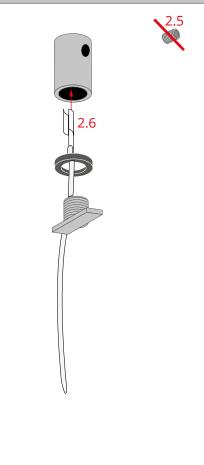
Unscrew the pressure screw (2.5) and the threaded mount lock (2.1), remove the o-ring (2.2) and the damaged connector wire (2.3) from the head (2.4).
