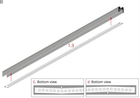
Adhere the LED tape (1.3) in the profile so as not to cover the holes (figures c, d).
