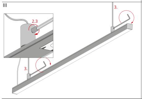
Insert the cables (3) into the heads and lock them by tightening the pressure screws (2.3).
