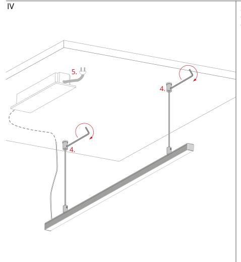
Suspend the lighting fixture from the ceiling fasteners (4) and connect the cable to the 12 V / 24 V power supply (5).
