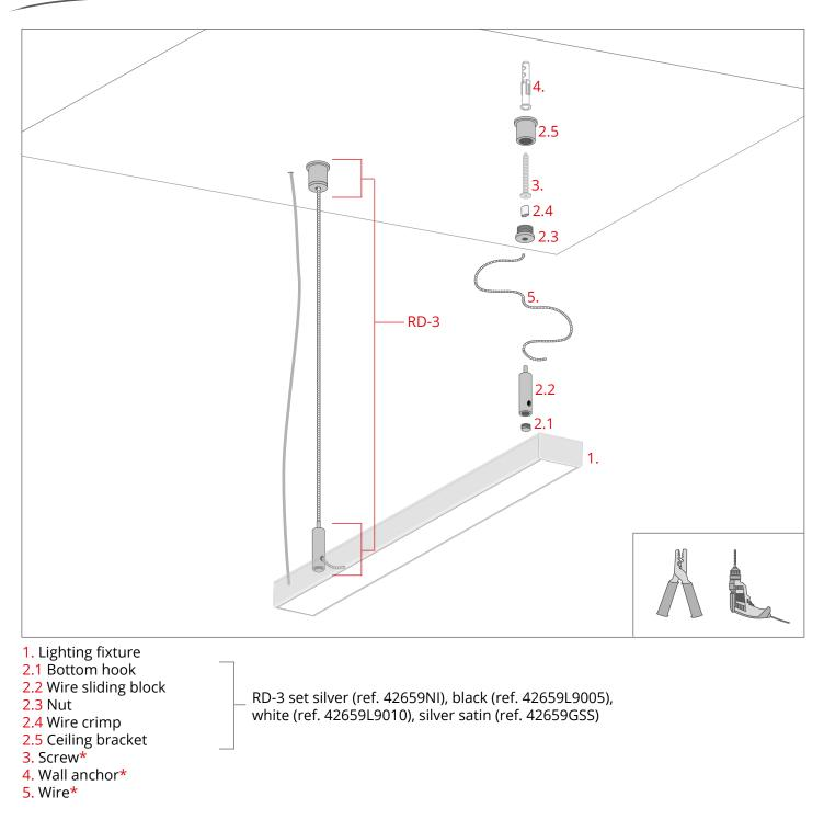
\*Wire, screws and wall anchors are not included in the RD-4 set. Commonly available screws ø 5 mm for a given type of surface should be used (wall, drywall, wood, sheet metal, etc.).
