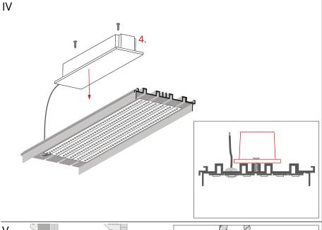
Mount the power supply (4) on the back of the extrusion.
