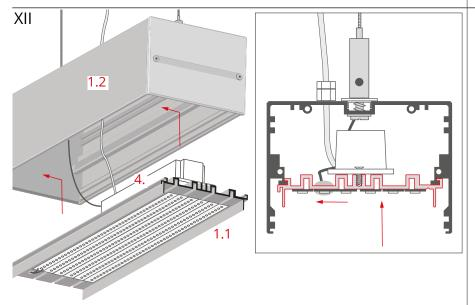
Connect the power supply (4) to the power cable.
