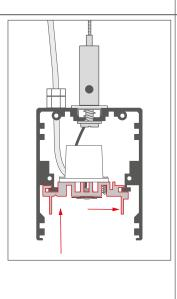
Connect the power supply (4) to the power cable.
