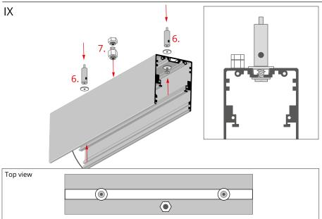
Attach the fasteners (6) and mount the metal gland (7).
