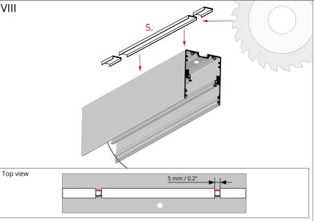
Attach the cover (5) between the holes for the fasteners leaving 5 mm space between the cover sections.
