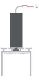
${\bf 5}_{ullet}$  Bend the power connector (E) so that it fits into the sleeve (B). Put an arm with thread through the connector and secure it with nuts (D, G) and a locking washer (F).
