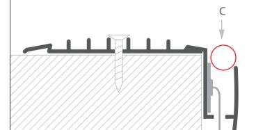
**5.** Glue the end cap (B) to the extrusion.
