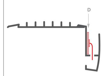
$\boldsymbol{2}_{\bullet}$  Fasten the extrusion (A) to the surface with appropriate screws for the substrate.
